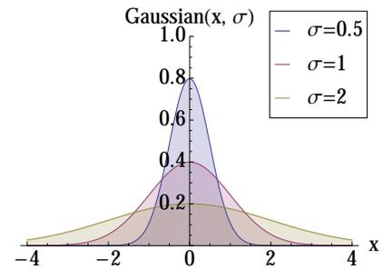
**Figure 1:** Three normal (or Gaussian) distributions each with a mean of zero but with differing values of  $\sigma$ , the standard deviation. Larger standard deviations indicate a greater spread in the distribution.
